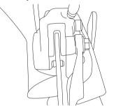
Each rear brake pad is provided with a wear indicator groove, which allows you to check the brake pad wear without having to disassemble the brake. Check the brake pad wear as follows.
