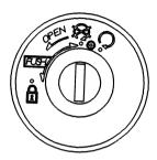
The main switch/steering lock controls the ignition and lighting systems, and is used to lock the steering. The various positions are described below.
