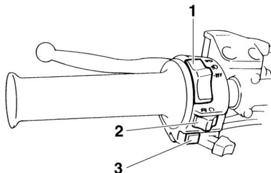
1. Interruptor de luces “ $\equiv \circ / \equiv \circ / \text{OFF}$ ”
